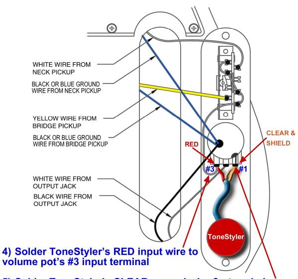
5) Solder ToneStyler's CLEAR ground wire & stranded copper shield wire to volume pot's #1 ground terminal or metal case
